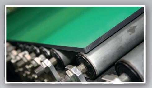
Ekon is the leading producer of polyethylene (PE) and polypropylene (PP) sheet and roll material through the flat-die-extrusion process. Other raw materials which can be processed are Biopolymers, Plastomers and TPE's. A combination of different raw materials by co-extrusion is another option.
